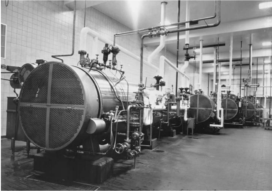
FIGURE 11.7 Continuous rotary sterilizer system. (Courtesy FMC Corporation.)
