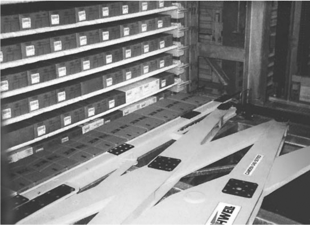
FIGURE 6.20 Plate contact freezing system. (Courtesy of Crepaco, Inc.)
