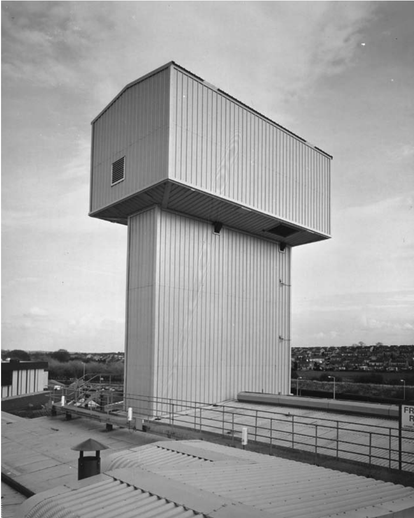
FIGURE 11.8 Exterior view of continuous hydrostatic sterilizer. (Courtesy FMC Corporation.)
